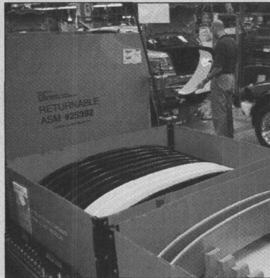
Returnable containers and dunnage can be made of plastic, corrugated or metal as seen at the Saturn plant in Wilmington, Delaware.
