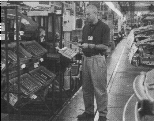
Line side inventory management and replacement are enhanced with containers and racks designed for JIT operations such as the Saturn plant in Wilmington, Delaware.
